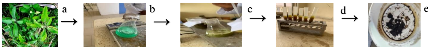
Figure 1: Scheme of synthesis of NiO Nanoparticles
