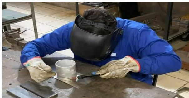
Figure 3 - Operator at the workstation performing a welding simulation.
