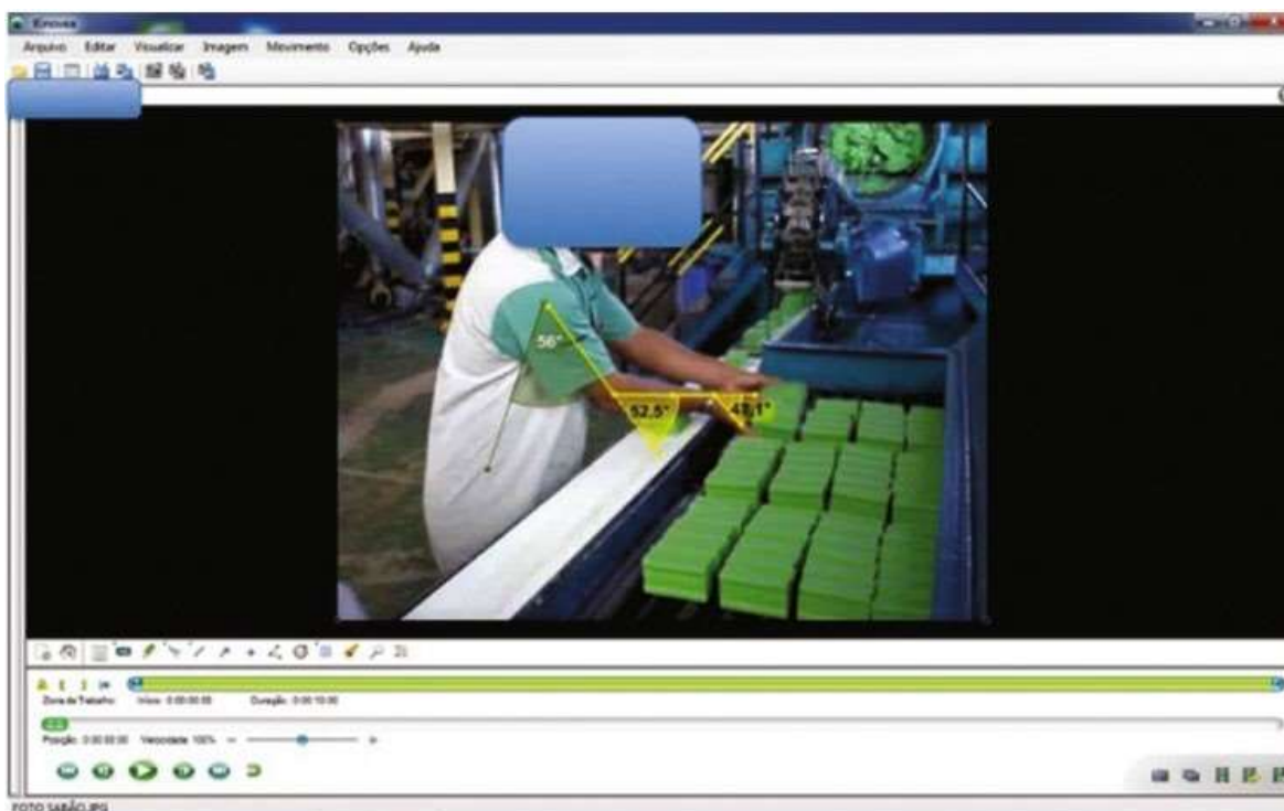
Figure 1. Kinovea Software in Biomechanical Analysis
