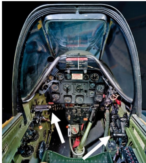
Figure 2 - Cockpit of a P-51D. The arrows show the power lever (left) and hood opening crank (right) Source: Adapted from Smithsonian (201?), with distribution permission CC0 (CC, 202?a)
