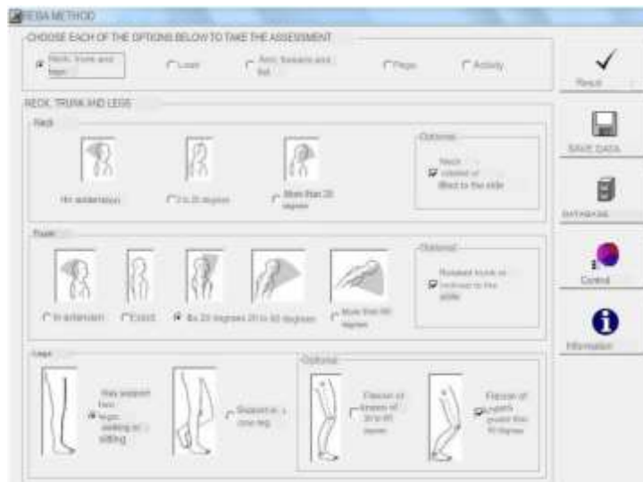
Figure 17 - Evaluation of the limbs: neck, trunk, and legs using the REBA method
