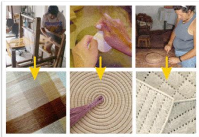
Figure 01: Techniques used in AALP sisal production: woven stitch, closed stitch and lace stitch.
