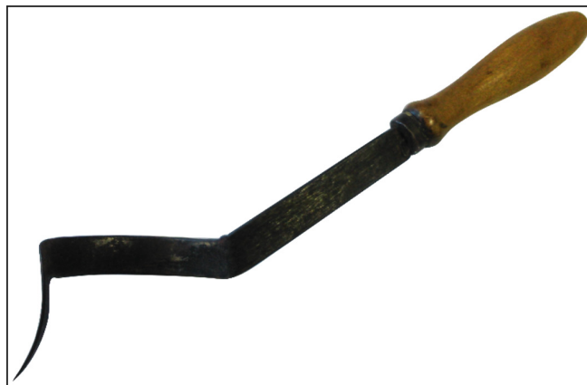
Figure 1. Banana tumbling tool. Source: The authors.
