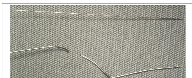
Figure 2 - Detail of spinal 27G Quincke Needle (B Braun<sup>®</sup>) Fractured at 43 mm of its tip and its Mandrel. Removed distal fragment after surgical exploration of Interspinous Ligament L<sub>2</sub>-L<sub>3</sub> Region
