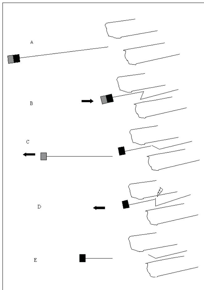
Figure 3 - Drawing showing Possible Needle Deformation (A, B and C) and Fracture (D and E) Mechanisms
