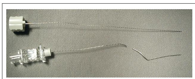
Figure 1 - Fractured Spinal 27G Quincke Needle and its respective Deformed Mandrel
