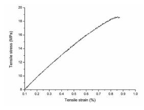
**Figure 2.** Representative tensile stress-strain curve of virgin PHB determined at 1 mm.min<sup>-1</sup> by using a universal machine Shimadzu AG-X 10kN model, based on the ISO standard 527-2. The test-specimens, type 5B, were prepared by laser cutting from films prepared by compression molding.
