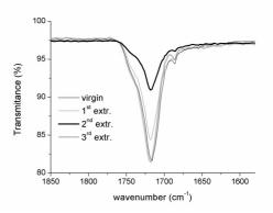
Figure 5. FTIR spectra in stretching region of -C=O of PHB before and after each extrusion cycle.
