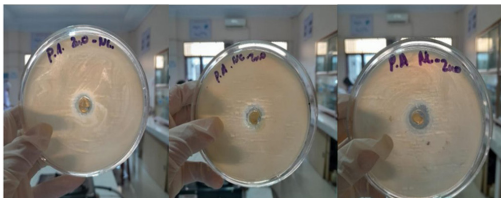
Figure 6. BC-ZnO antibacterial activity test against Propionibacterium acnes .
