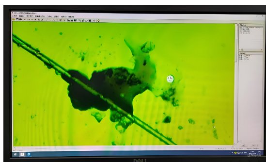
Figure 5. The interaction of fiber from the fly ash of thermal power plants with road asphalt bitumen.
