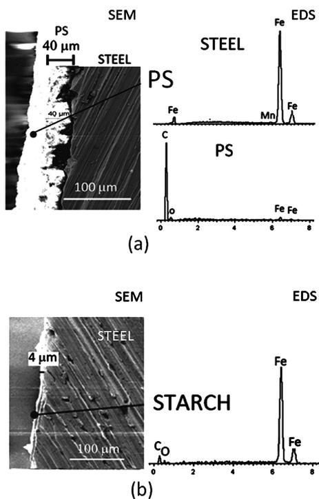
**Figure 3.** (a) Photomicrography for secondary electrons 600× substrate profile (SEM) of anticorrosive film of polystyrene (PS) on ASTM 1080 steel (Steel) and the energy-dispersive X-ray spectroscopy spectrum (EDS) for ASTM 1080 steel (Steel) and polystyrene (PS); (b) photomicrography for secondary electrons 600× substrate profile (SEM) of anticorrosive film of starch (Starch) on ASTM 1080 steel (Steel) and the energy-dispersive X-ray spectroscopy (EDS) only to the spectrum for starch.
