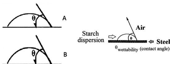
**Figure 1.** Schematic contact angle dynamics of (A) polystyrene coating fluid on steel and (B) the starch coating fluid on steel.
