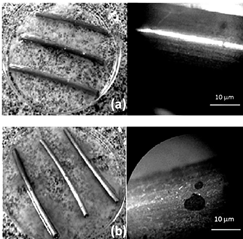
**Figure 2.** (a) Visual outcome by optical microscopy of the surface of the steel with polystyrene (PS) coating after a six-month saline test for corrosion; (b) visual outcome by optical microscopy of the surface of the steel with starch after 2 weeks of analysis of saline corrosion.
