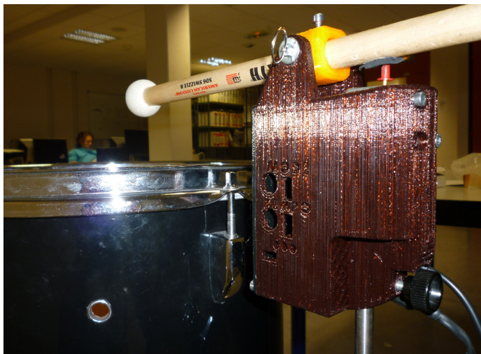
Figure 6. Final version of the MEM using the Rep/Rap manufacturing process.
