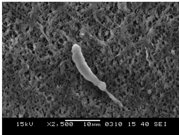
Figure 6 SEM-Portex Flat Filter, P. aeruginosa 2500× magnification, after bacterial infusion.
