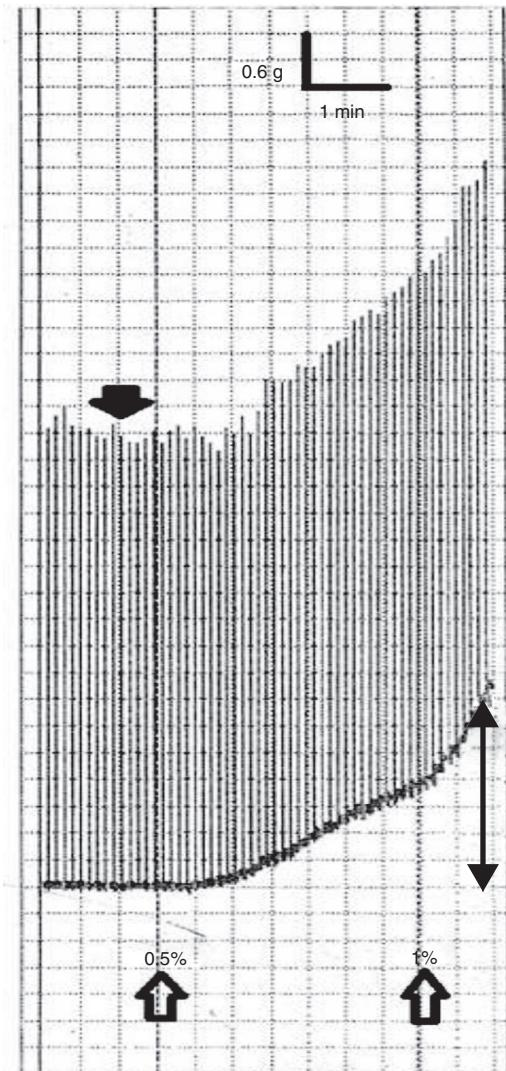
**Figure 1** *In vitro* muscle contracture test (IVCT) in response to halothane. The two lower arrows indicate the time at which the drug was added. The upper arrow indicates the lines that correspond to muscle contractions triggered by electrical stimulation. The lateral double arrow indicates the ascension of the base line, which corresponds to an abnormal muscle contracture.
