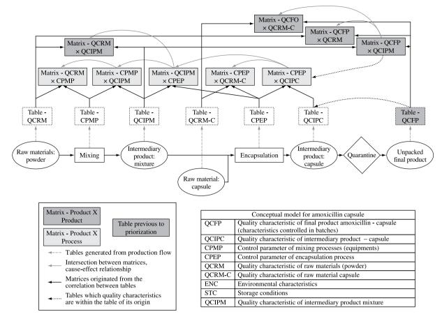
Figure 2. The construction logic of a conceptual model for amoxicillin-capsule.
