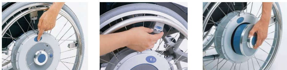
Figure 9: Selecting the potency, the sensibility and dismounting the batteries' E-motion.
