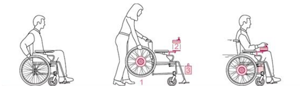
Figure 7: Substitute the two rear wheels for two motorized ones.
