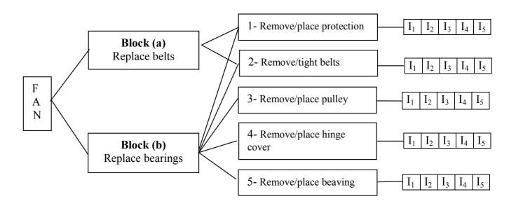
Figure 7 — Support tree with diagram of disassembly/assembly activities to "replace belts and beavings".
