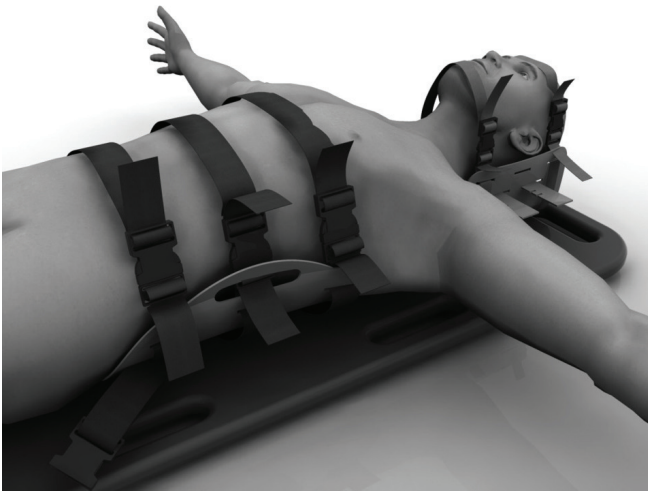
Figure 5. Concept of immobilization device coupled to the patient and to the backboard.
