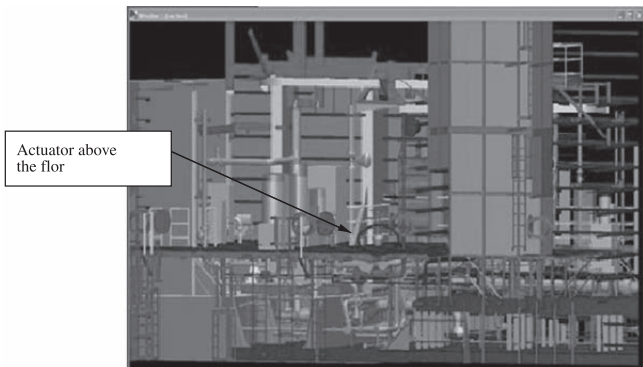
Figure 4. 3D Model inconsistency, verified in design review section.
