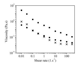
**Figure 6.** Steady-state viscosity versus shear rate for CNF ( $\bullet$ ), CNC-n (X) and CNC-t ( $\bullet$ ) suspensions with concentration of 0.6 wt%.
