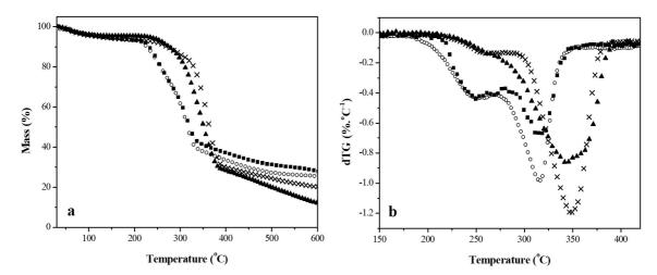
Figure 4. (a) TGA and (b) dTG curves for: CP (▲), CNC-n (X), CNC-t (o) and CNF (■).
