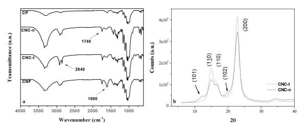
Figure 3. FTIR (a) spectra for paper and nanocellulosic materials and XRD (b) patterns for CNC-t and CNC-n.
