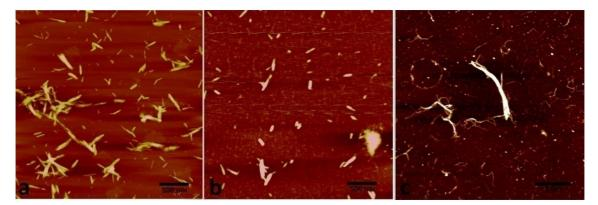
Figure 2. AFM images of (a) CNC-n, (b) CNC-t and (c) CNF.
