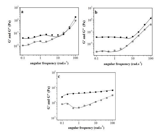
Figure 7. Storage, G' (solid symbols) and loss, G" (empty symbols) moduli as a function of oscilation frequency for (a) CNC-t, (b) CNC-n and (c) CNF.
