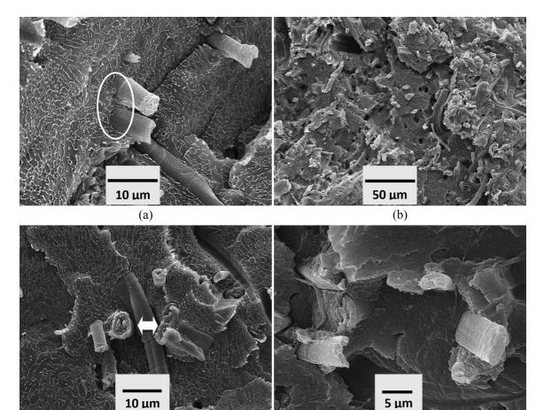
**Figure 7.** SEM micrographs of the cryogenic fracture surface of injection molded composites: (a) HDPE/20EVA20CF showing fiber-matrix interaction and co-continuous EVA phase, (b) HDPE/30EVA20CF showing the homogeneous distribution of the fibers, (c) HDPE/40EVA20CF highlighting fiber diameter and (d) HDPE/40EVA20CF composite after extraction with acetone with higher magnification.
