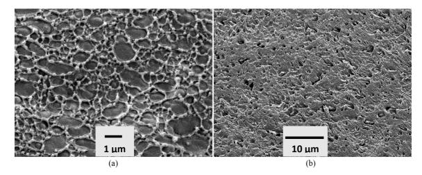
Figure 4. SEM micrographs of the fracture surface of injection molded blends: (a) HDPE/30 EVA with scale bar of 1  $\mu$ m and (b) HDPE/40EVA after extraction with acetone with scale bar of 10  $\mu$ m.
