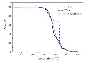
Figure 2. Comparison of the thermogravimetric curves of HDPE, EVA and the blend HDPE/20EVA, measured under synthetic air flow at 10 °C min<sup>-1</sup>.
