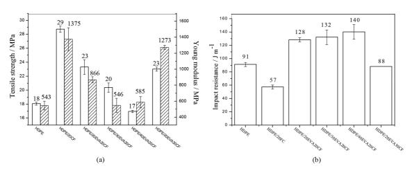
Figure 10. Comparison of the mechanical properties of pure HDPE, HDPE/20CF composite and composites of blends with different EVA and CF contents in wt. %: a) tensile strength and Young's modulus and b) impact resistance.
