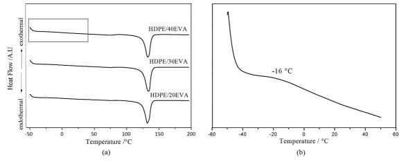
Figure 1. a) DSC curves (2<sup>nd</sup> heating) of HDPE blends with 20, 30 and 40 wt. % of EVA and (b) detail of the part of the curve used for  $T_{a}$  determination in a) for HDPE/40EVA. Curves in a) were vertically shifted for better comparison.
