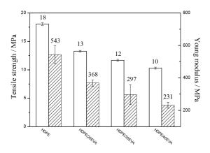
**Figure 6.** Comparison of tensile strength **and** Young modulus **COMPARENT OF EVA** blends, as a function of EVA content.
