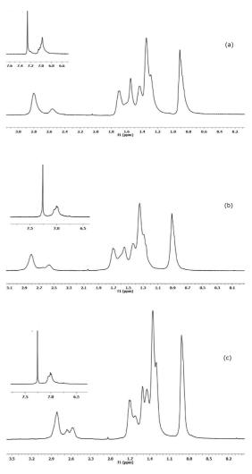
**Figure 2.** <sup>1</sup>H-NMR spectra of (a) PHTcl; (b) PHTdcm16; (c) PHTdcm40 with expanded area corresponding to the region of aromatic hydrogens.
