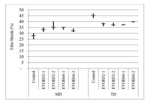
Figure 5. Machine (MD) and Transverse Directions (TD) shrink of EVOH and PVDC (control) multilayer shrinkable films. Control: EVA/tie/PVDC/tie/LLDPE; EVOH32-1: PET/tie/Ionomer/tie/ PA6/66+aPA/EVOH 32 mol%/tie/LMDPE/LLDPE; EVOH32-2: PET/tie/Ionomer/tie/PA 6/66+aPA/EVOH 32 mol%/PA6/66+aPA/ tie/LLDPE; EVOH44-1: PET/tie/Ionomer/tie/PA6/66+aPA/EVOH 44 mol%/tie/LMDPE/LLDPE; EVOH44-2: PET/tie/Ionomer/tie/ PA 6/66+aPA/EVOH 44 mol%/PA6/66+aPA/tie/LLDPE.
