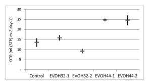
Figure 4. Oxygen transmission rate at 23 °C and 75% RH of EVOH and PVDC (control) multilayer shrinkable films. Control: EVA/tie/PVDC/tie/LLDPE; EVOH32-1: PET/tie/Ionomer/tie/ PA6/66+aPA/EVOH 32 mol%/tie/LMDPE/LLDPE; EVOH32-2: PET/tie/Ionomer/tie/PA6/66+aPA/EVOH 32 mol%/PA6/66+aPA/ tie/LLDPE; EVOH44-1: PET/tie/Ionomer/tie/PA6/66+aPA/EVOH 44 mol%/tie/LMDPE/LLDPE; EVOH44-2: PET/tie/Ionomer/tie/ PA6/66+aPA/EVOH 44 mol%/PA6/66+aPA/tie/LLDPE.
