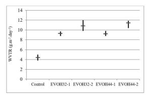
Figure 3. Water vapour transmission rate of EVOH and PVDC (control) multilayer shrinkable films. Control: EVA/tie/PVDC/ tie/LLDPE; EVOH32-1: PET/tie/Ionomer/tie/PA 6/66+aPA/ EVOH 32 mol%/tie/LMDPE/LLDPE; EVOH32-2: PET/tie/ Ionomer/tie/PA6/66+aPA/EVOH 32 mol%/PA6/66+aPA/tie/ LLDPE; EVOH44-1: PET/tie/Ionomer/tie/PA6/66+aPA/EVOH 44 mol%/tie/LMDPE/LLDPE; EVOH44-2: PET/tie/Ionomer/tie/ PA6/66+aPA/EVOH 44 mol%/PA6/66+aPA/tie/LLDPE.
