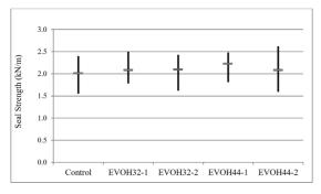
Figure 1. Bottom seal strength at yield of EVOH and PVDC (control) multilayer shrinkable films. Control: EVA/tie/PVDC/ tie/LLDPE. EVOH32-1: PET/tie/Ionomer/tie/PA6/66+aPA/ EVOH 32 mol%/tie/LMDPE/LLDPE; EVOH32-2: PET/tie/ Ionomer/tie/PA6/66+aPA/EVOH 32 mol%/PA6/66+aPA/tie/ LLDPE; EVOH44-1: PET/tie/Ionomer/tie/PA6/66+aPA/EVOH 44 mol%/tie/LMDPE/LLDPE; EVOH44-2: PET/tie/Ionomer/tie/ PA6/66+aPA/EVOH 44 mol%/PA6/66+aPA/tie/LLDPE.
