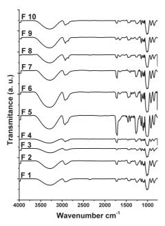
Figure 5. FT-IR analysis of the starch-PVA biodegradable sheets (F1-F10, formulations according to Table 1).
