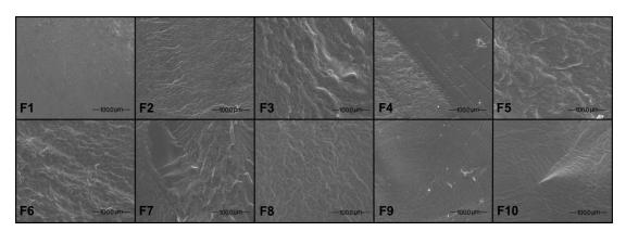
Figure 4. Scanning electron microscopy micrographs of the fracture of the sheets with magnification at 800 x (F1-F10, formulations according to Table 1).
