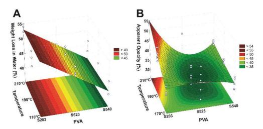
Figure 2. Surface response plot for weight loss in water – WLW (A) and apparent opacity (B) of the biodegradable sheets.
